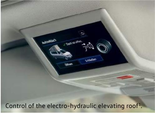
Control of the electro-hydraulic elevating roof<sup>1</sup>.
